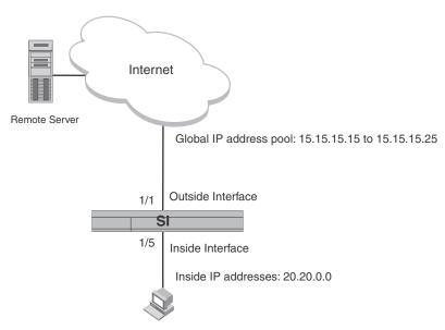
This example requires that Interfaces 1/5 and 1/1 be configured as inside and Outside interfaces respectively as shown.
